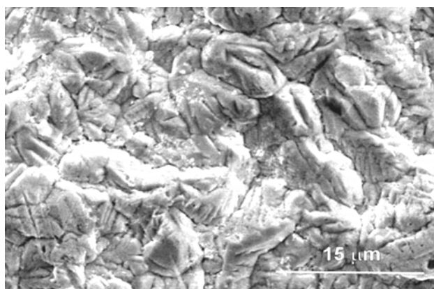
Figure 3. Microstructure of composite electrode Pb-Ti-0.55%. Magnification x2000.
